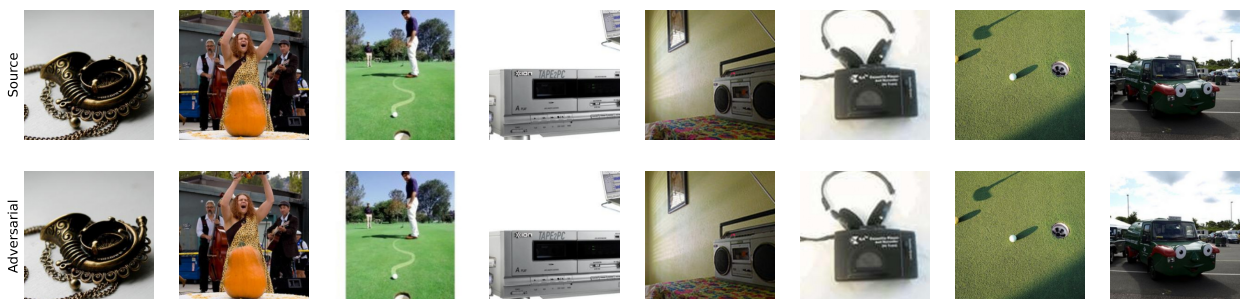
Figure 12. Adversarial samples and their source images crafted with IIW attack with \epsilon = 0.32143 , with low LPIPS scores between the source and the resulting adversarial sample ( d_{\text{lpiips}} < 0.2 ).
